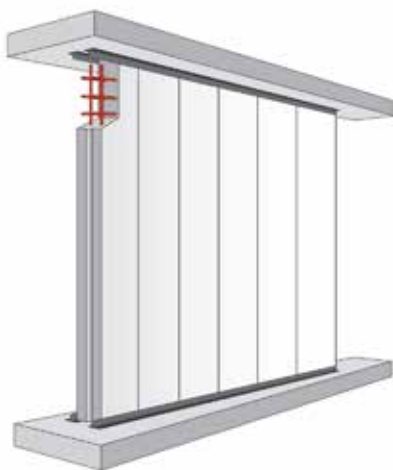
EBLOCK Panel installed vertically
